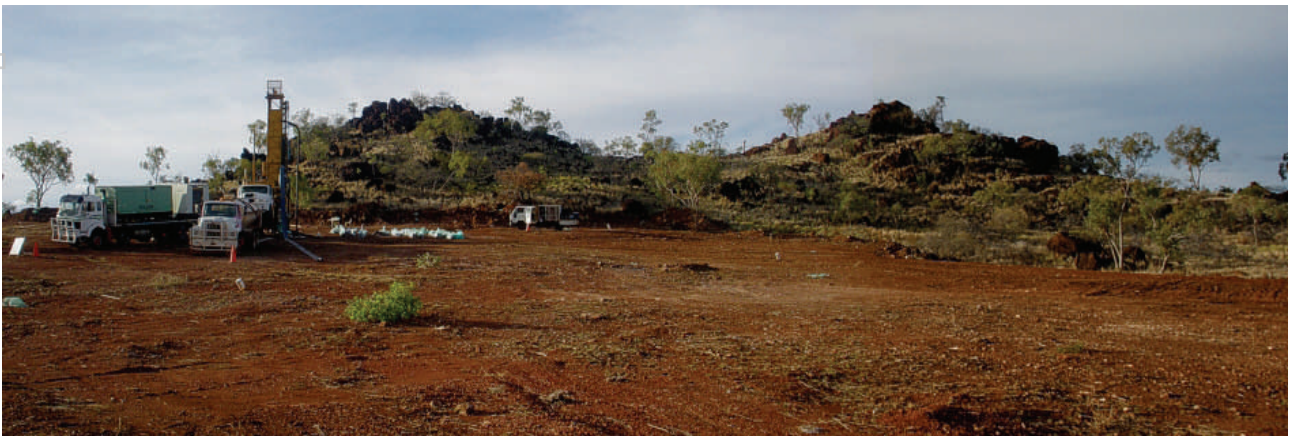
Fig 3: Recent RC programme drilling vertical holes to 50m depth, to test the zone beneath the shallow high-grade bedrock results.
