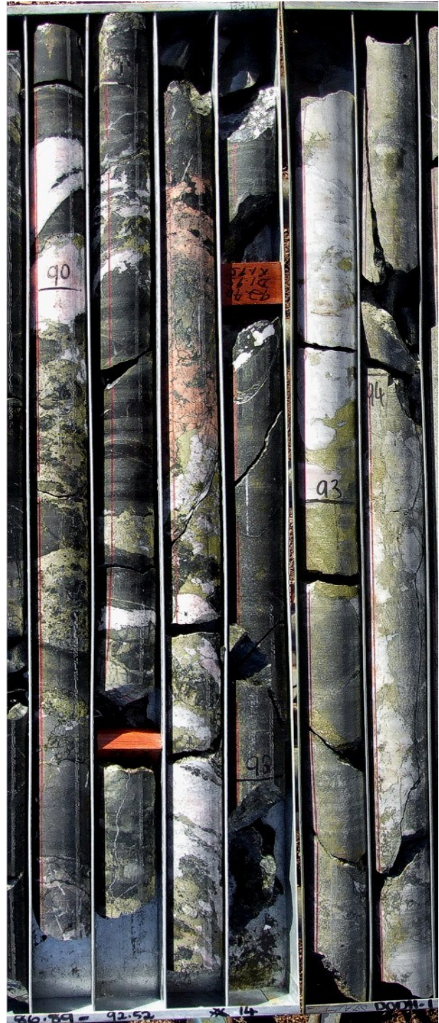
Fig 3: Example of mineralisation in diamond drill hole DODH122, which intersected several high grade shallow zones in areas estimated to be low grade by the resource estimation block model. The intersection above shows the interval from approximately 89-94m down-hole depth, which assayed 5m @ 3.28% CuEq.
