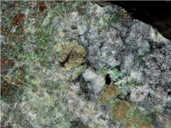
Fig 3: visible gold associated with highly-altered zone intersected in diamond drill hole DODH240, from 7 - 20m (photos from approximately 11m).
