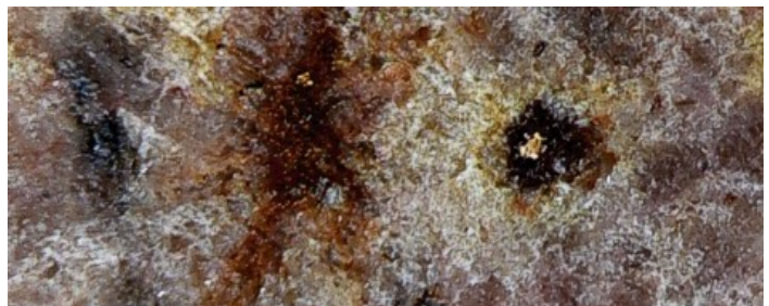
Fig 5: Disseminated visible grains of gold and possible rare native tellurium associated with highly-altered zone intersected in diamond drill hole DODH240m from 7 - 20m (photos from approximately 11m)
