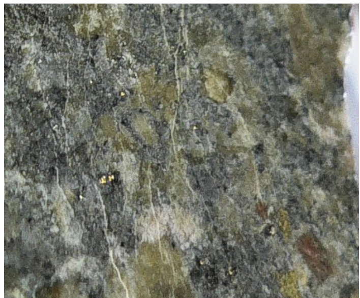
Fig 6 Disseminated visible grains of gold and possible rare native tellurium associated with highly-altered zone intersected in diamond drill hole DODH240m from 7 - 20m (photos from approximately 11m).
