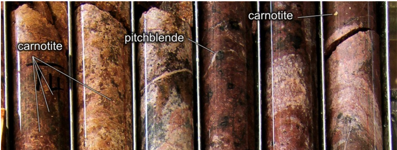
Fig 4. Diamond drill hole DODH251 with uranium minerals carnotite and pitchblende throughout (approximately 14 - 18.5m shown).
