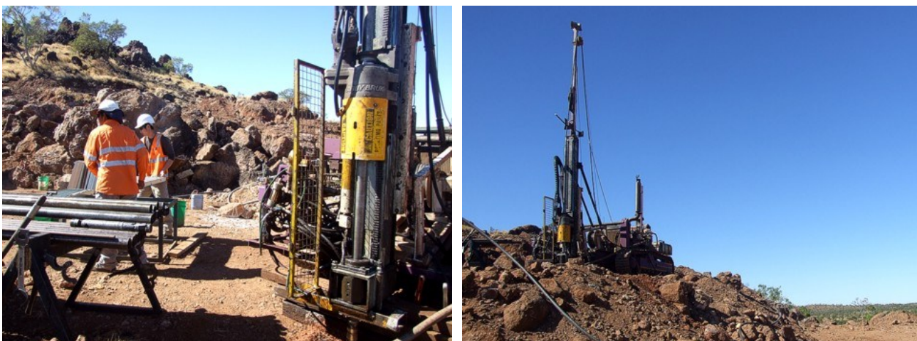
Fig 5. Recovering drill core trays from diamond rig at Wilgar (left), and diamond rig on cleared drilling platform highlights the difficult terrain at the prospect.
