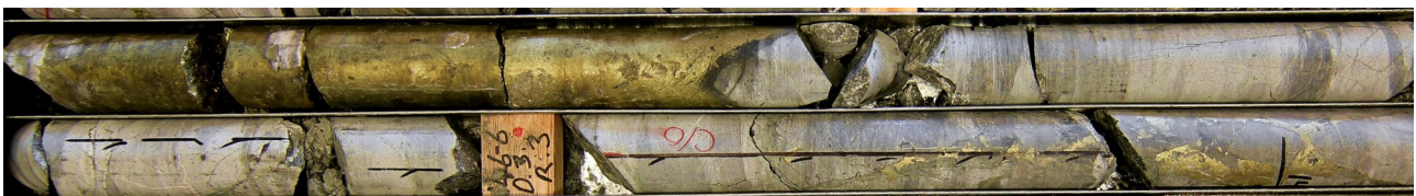
Figure 2: Massive sulphides intersected at approximately 145m in diamond drill hole DODH255.
