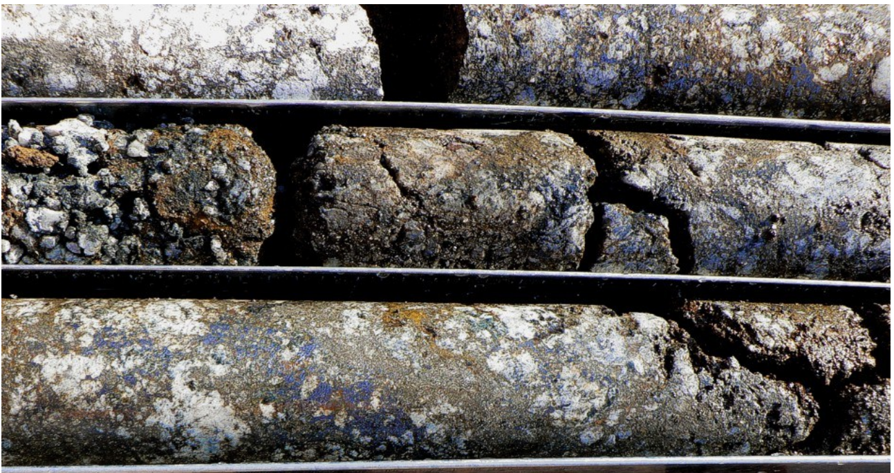
Figure 1: Semi-massive chalcocite and pyrite infill of quartz-breccia at approximately 65m in DODH320.
