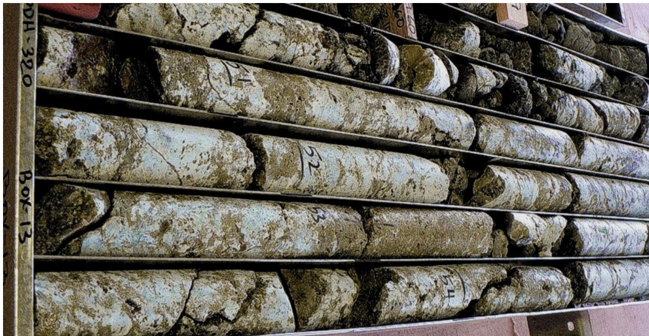
Figure 2: Semi-massive chalcocite (copper mineral = 79.85% Cu) and pyrite infill, of quartz-breccia intersected in diamond drill hole DODH320 - approximately 49.5-54.5m shown.
