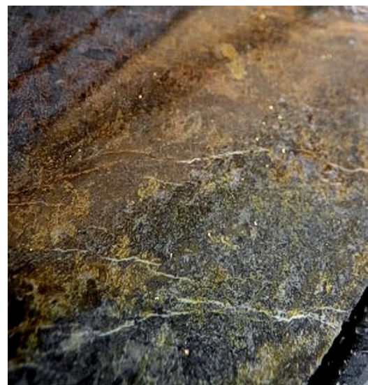
Figure 4: visible gold in diamond drill hole DODH223, which assayed 655g/t Au at 17m.
