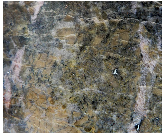
Figure 3: visible gold and possible gold-tellurides in diamond drill hole DODH240 which assayed 348g/t Au at approximately 11m).
