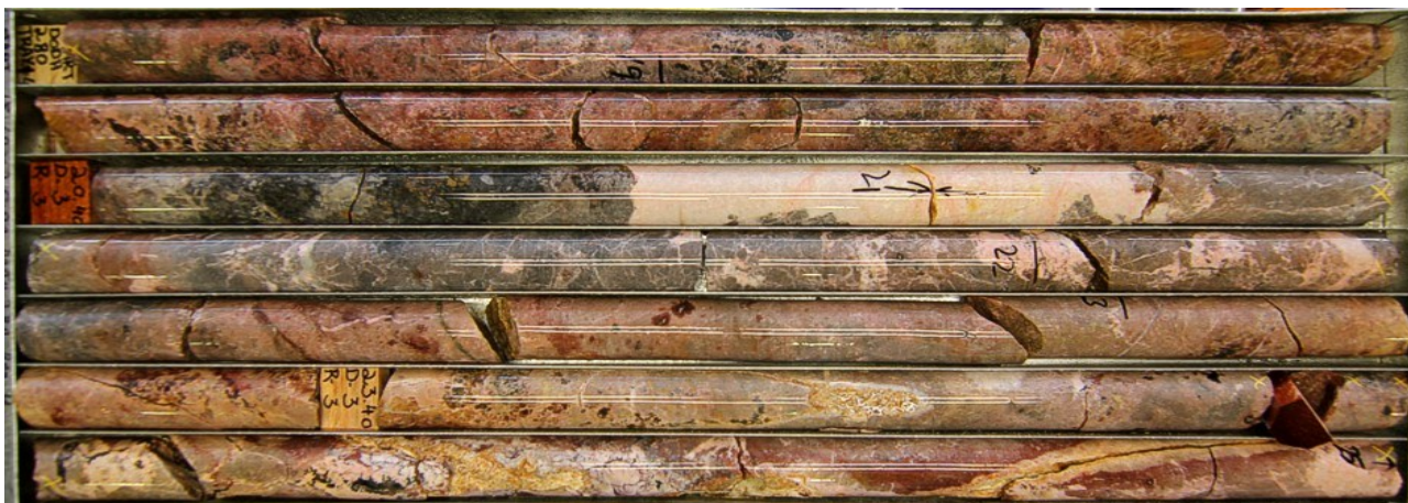
Figure 5: DODH280 from 18.6 - 25m, showing altered and mineralised drill core.
