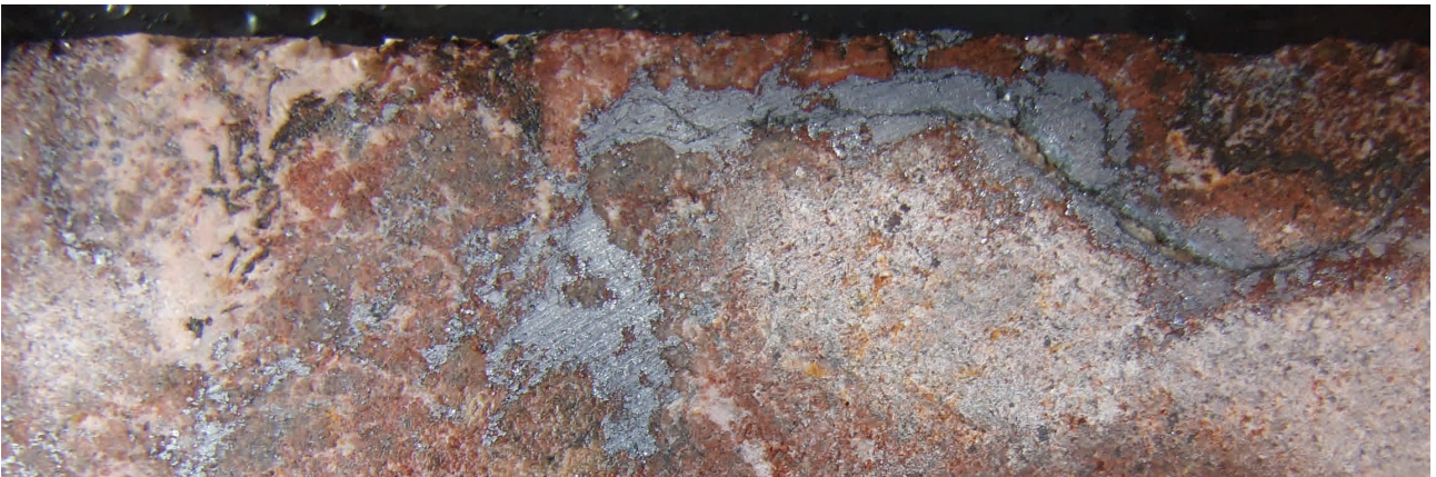
Figure 1: Visible drysdallite (molybdenum mineral) in diamond drill hole DODH314 at approximately 27m, assay results for 27-28m 2.26% Mo, 5.28g/t Au, 400g/t Ag and 249ppm Te.
