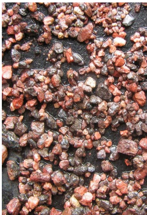
Figure 3: LMRC754 - RC drill chips (wet) at 53m
