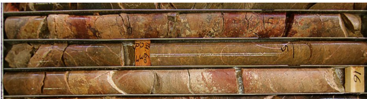
Figure 3: Diamond drill core from DODH304, from approximately 13-16m, which assayed 3m at 15.5 g/t AuEq. Visible gold was not observed.
