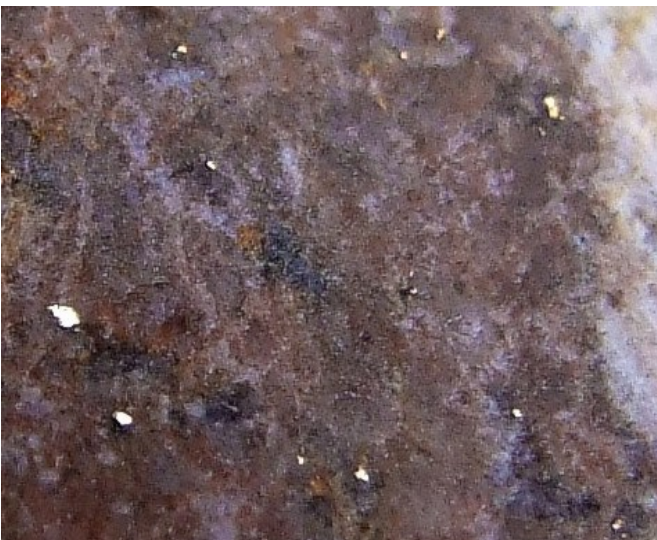
Figure 1: Visible gold in diamond drill hole DODH330 at approximately 19m. The 1m interval from 19-20m assayed 402g/t Au, 159g/t Ag, 1620ppm Te and 2140ppm U.
