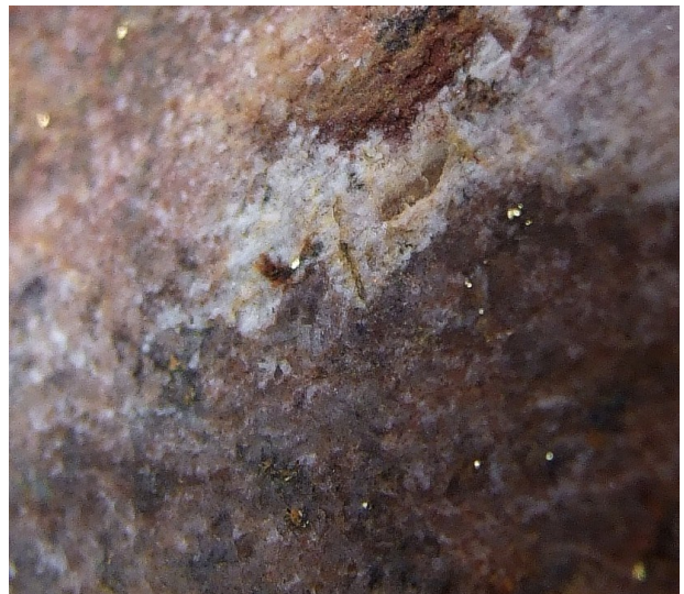
Figure 1: Visible gold in diamond drill hole DODH330 at approximately 19m. The 1m interval from 19-20m assayed 402g/t Au, 159g/t Ag, 1620ppm Te and 2140ppm U.
