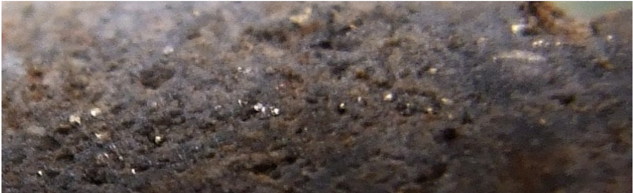
Figure 2: Visible gold in DODH330 at approximately 19m, assay for 19-20m 402g/t Au, 159g/t Ag, 1620ppm Te and 2140ppm U.
