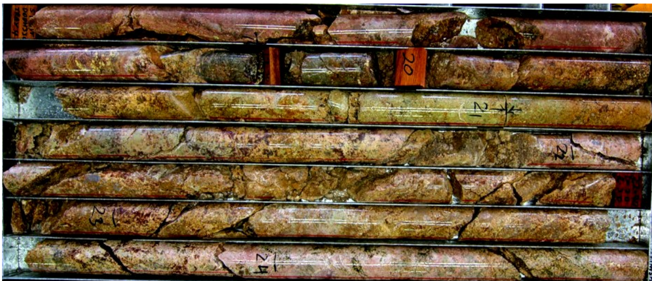
Figure 2: High-grade mineralised zone in diamond drill hole DODH330 from 18.7-24.6m, assay results for 18-25m 99.2g/t Au, 151g/t Ag, 534ppm and 1450ppm U.
