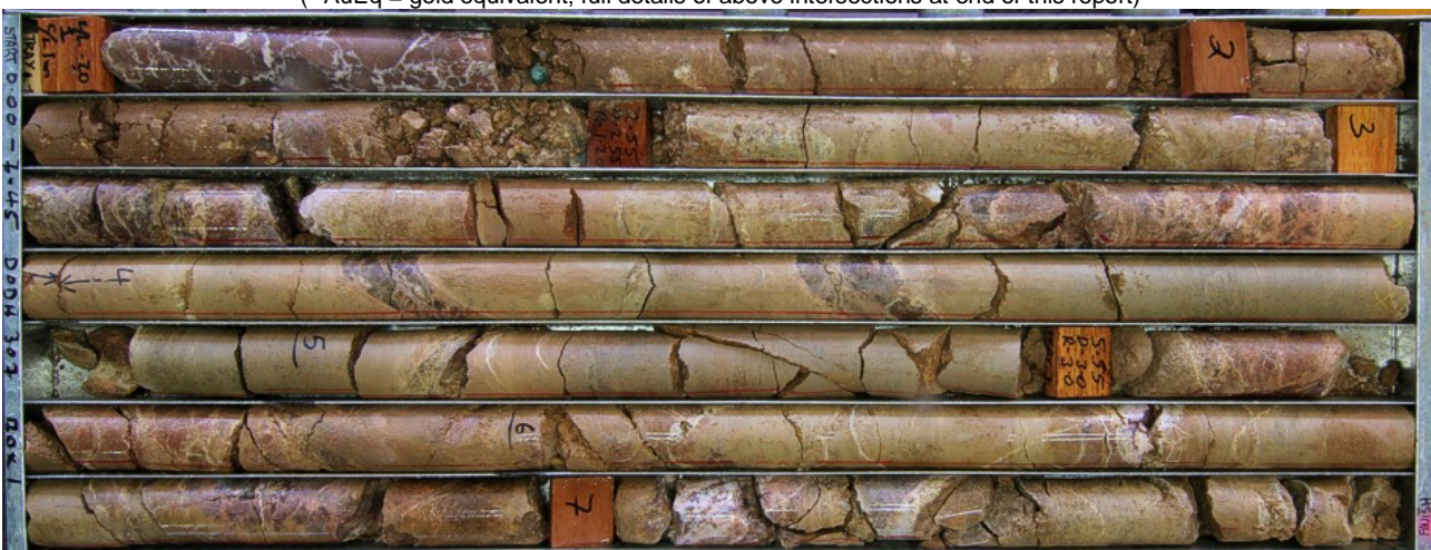
Figure 1: drill core from diamond drill hole DODH308, which assayed 7m @ 6.55g/t AuEq, from 1-8m
