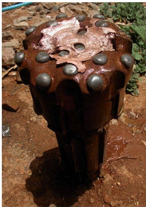
Fig 04 - Part of Native Copper Nugget caught in RC drill bit...
